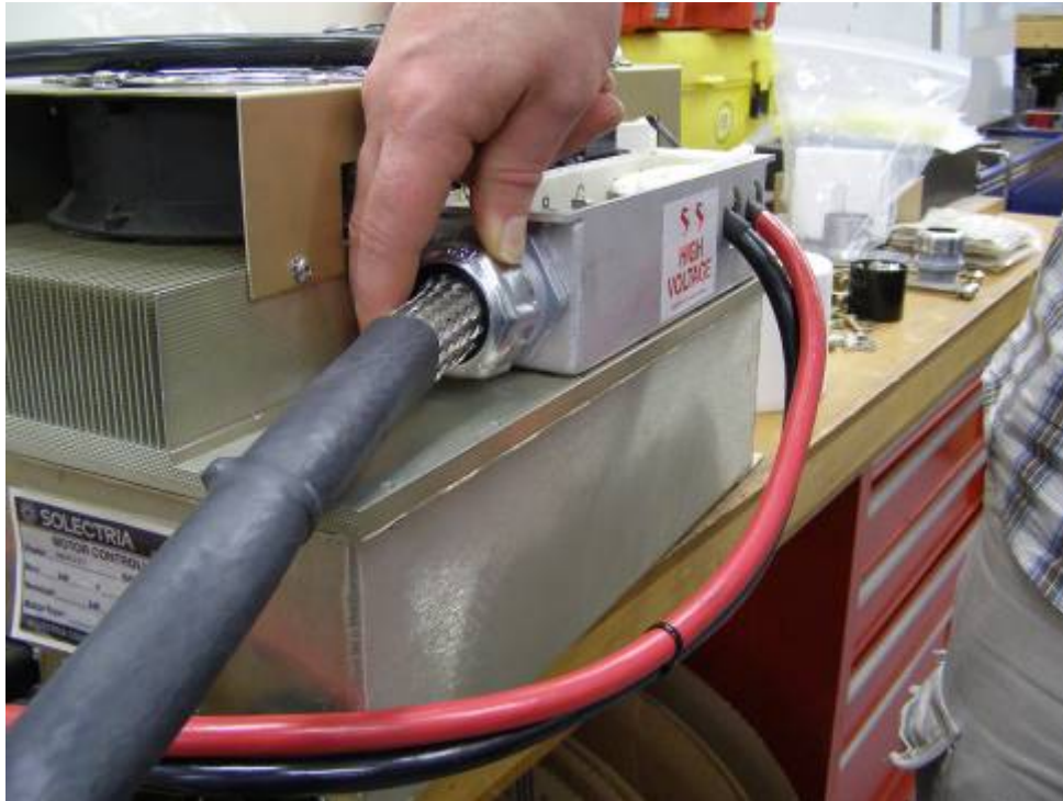
Figure 9. Screw on entrance fitting cap (nut) with black plastic flange washer underneath cap.
