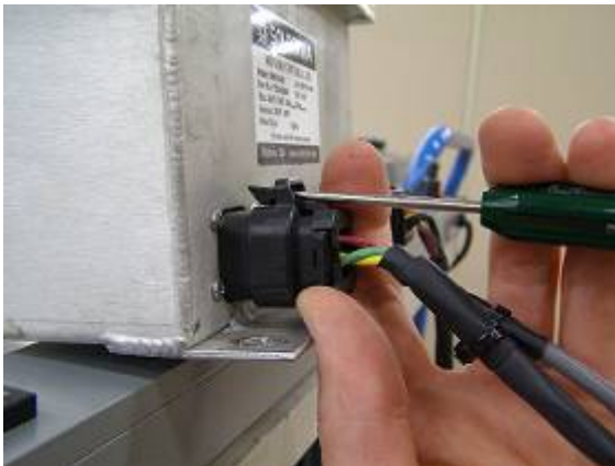
Figure 1. Removing 8-Pin “Comm.” Connector.
