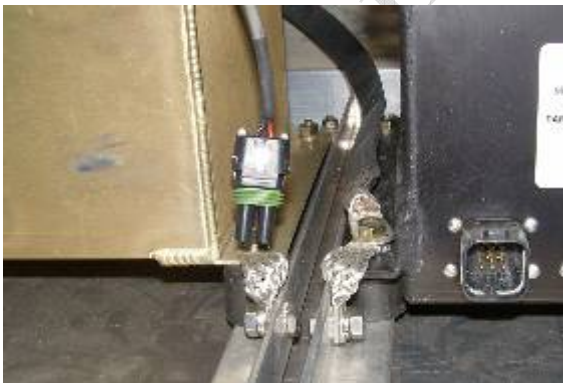
Figure 10. Example of the DMOC Grounding Strap Connection.
