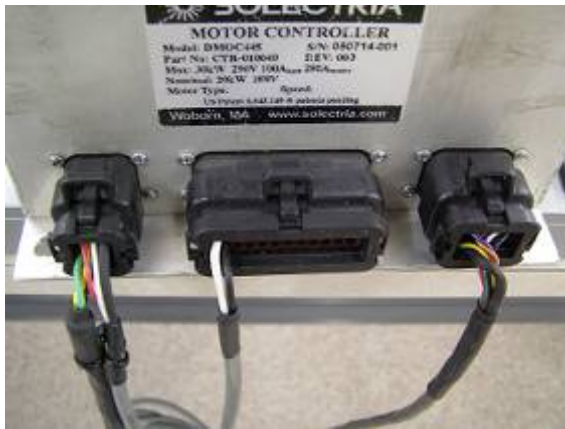
Figure 2. All three DMOC connectors in the position.
