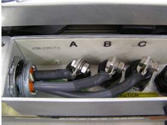
Figure 3. Motor Terminals.
