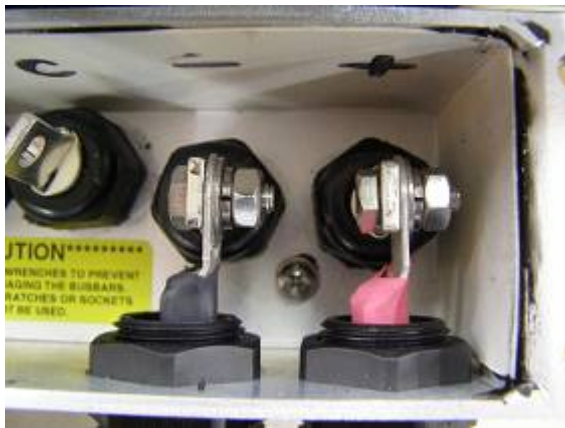
Figure 6. High Voltage Battery Terminals
