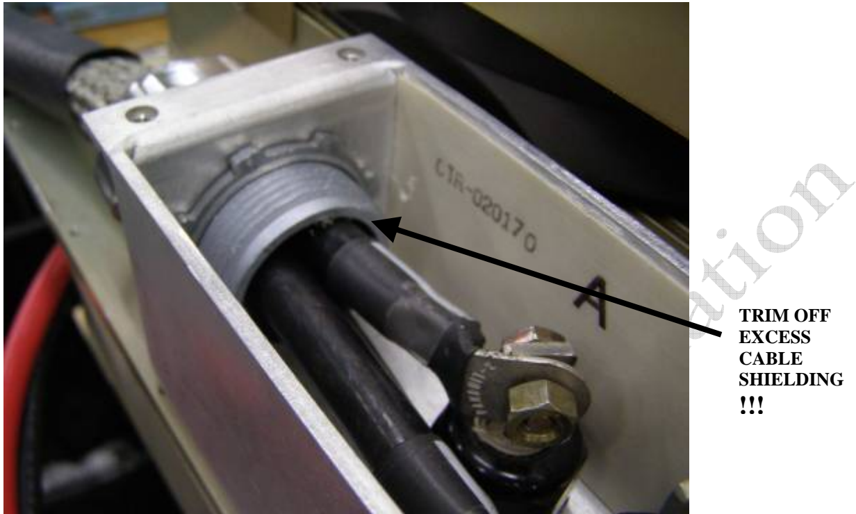
Figure 8. Trim off excess cable shielding inside terminal box. If excess cable shielding makes contact with DMOC AC terminals then a shock hazard will be created. Make sure that no shielding enters into terminal box.
