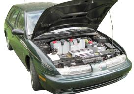
**Is it a hybrid?** No, it's a plug-in electric vehicle -- no gasoline. This means the only source of power is the on-board battery pack. When the battery pack goes dead, the car needs to be plugged in and recharged.
